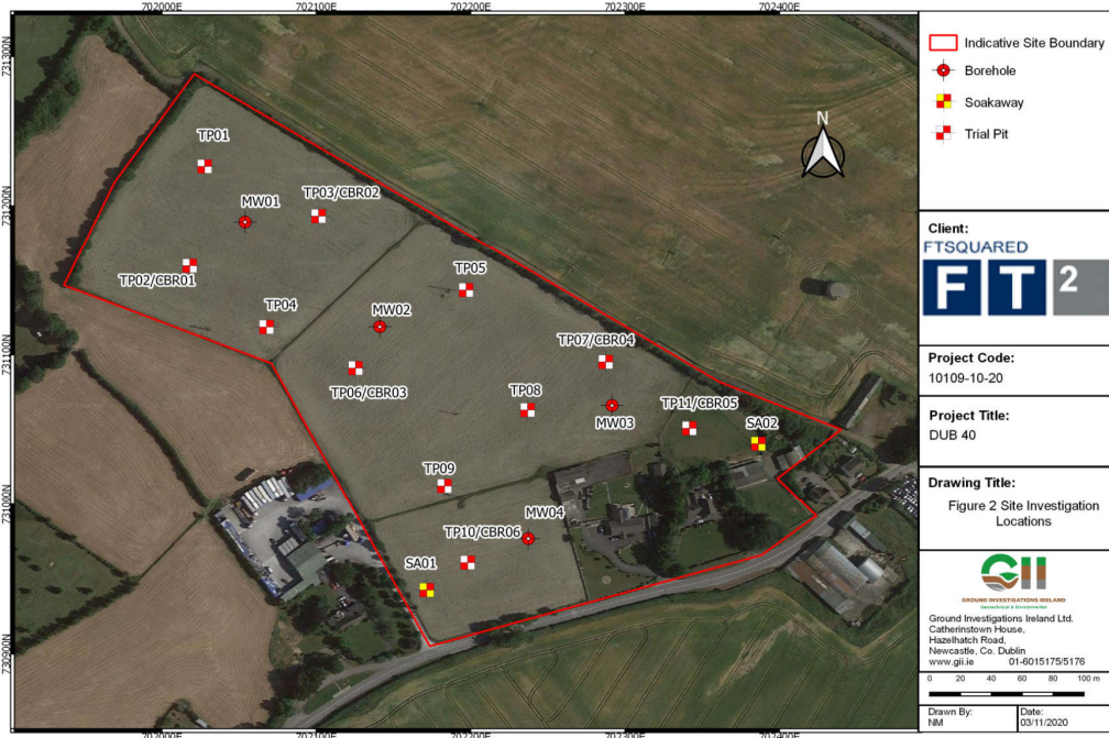
Figure 7.3 Site Investigation Locations (Source: GII, 2020). Redline boundary refers to the Site Investigation works and not the application redline boundary.
