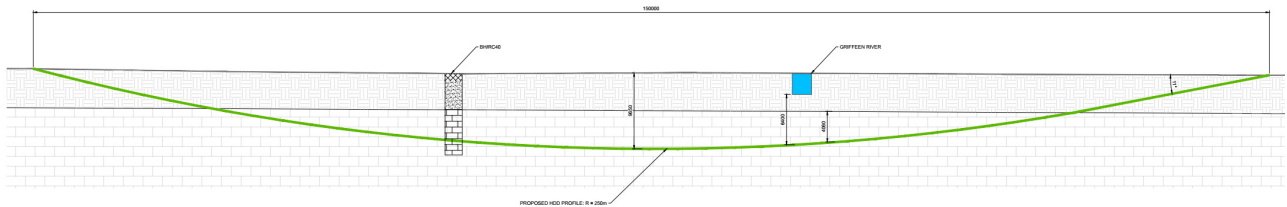
Figure 2.5 Typical cross-section of HDD profile under the Griffeen River (Source: Drawing no. 20_147-CSE-GEN-00-XX-DR-C-2130, CSEA Consulting Engineers)
